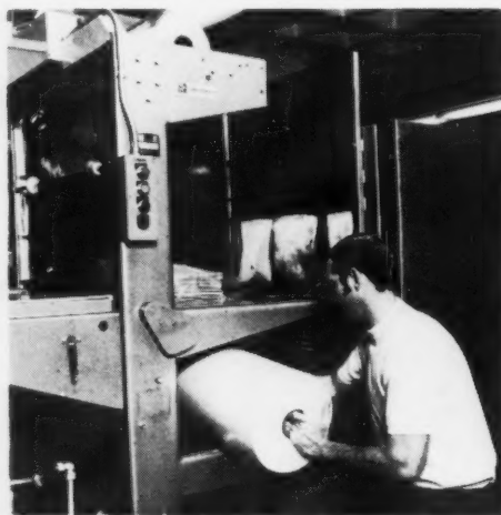
A roll of Polyfilm 303 shrink film is changed in 30 seconds by one man. Wire bundling required two men, five minutes, and special equipment to change wire bundles.
